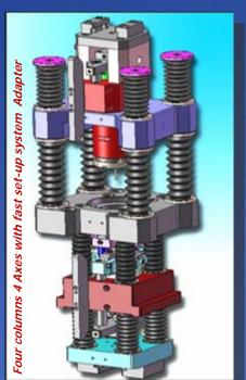
**Proment's** adapters include all hydraulic, pneumatic, digital readouts and other indicating equipment needs. We use Leather made bellow covers and metal treatments to ensure long lasting and trouble free tools.
